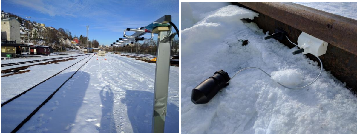
Figure 25 Antenna coverage field-test with sensors covered by snow
