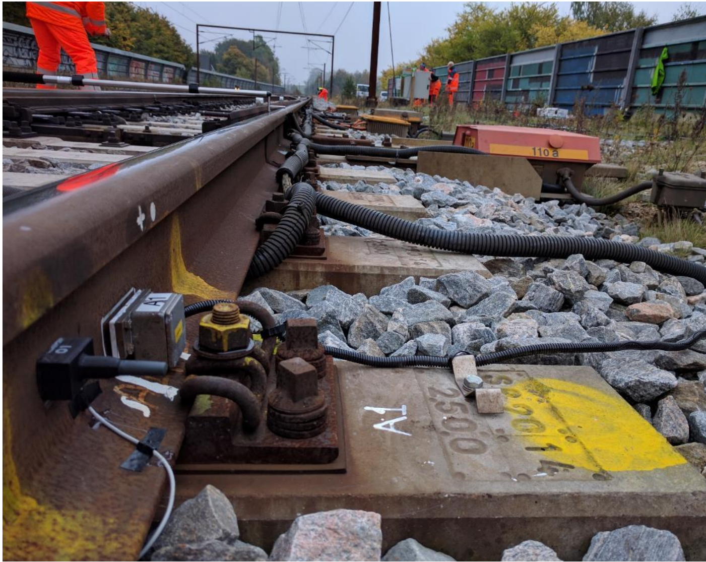
Figure C2 Sensor on the rail web
