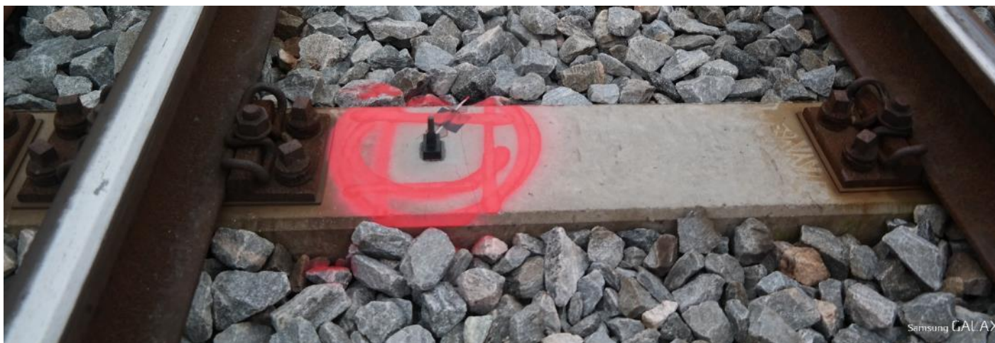
Figure C5 Sensor on sleeper
