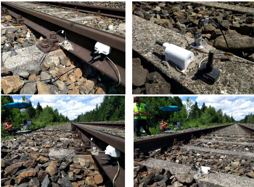
Figure 28 System test in Munich – sensors mounted on rail and sleeper
