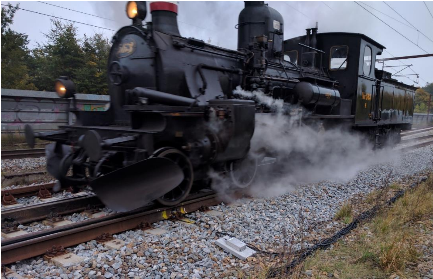
Figure C7 Test passage over the wireless sensors
