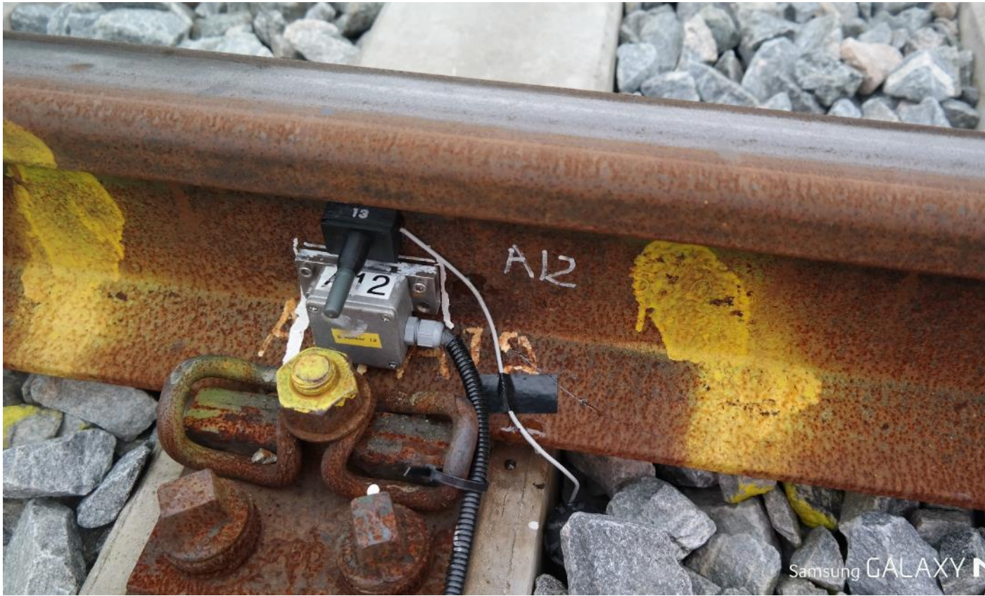
Figure C3 Sensor on the rail web
