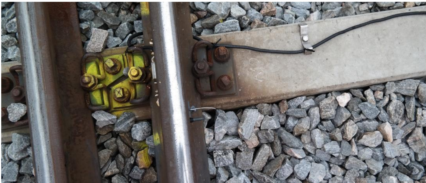
Figure C4 Sensor on the rail web (top view)
