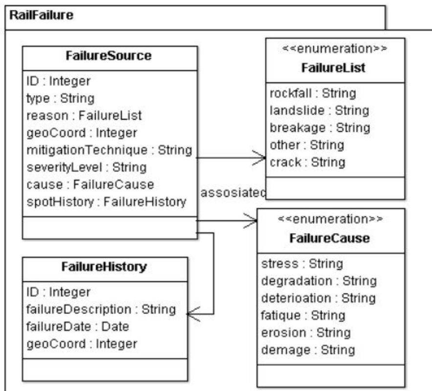
**Figure 7: Information Model (Rail Failure)**
