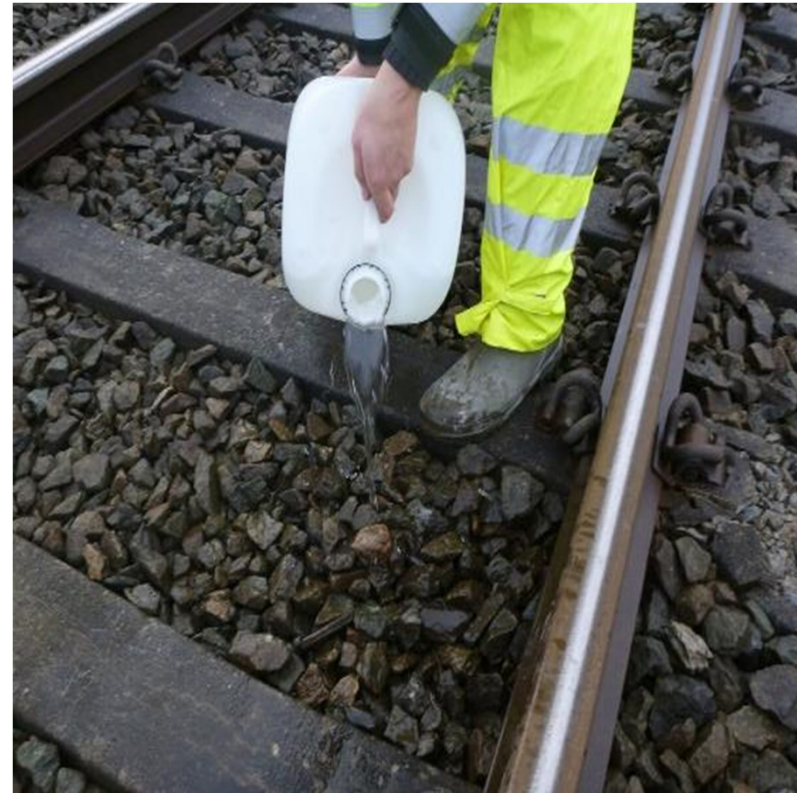
Water being poured continuously for the measurement
