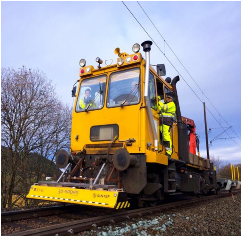
GPR mounted in Robel for on the field test
