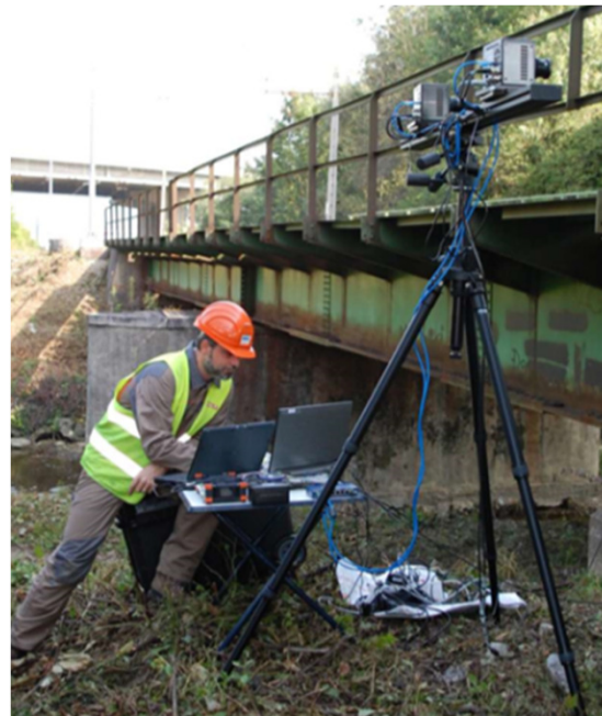
Railway track stiffness measurements, Slovenia
